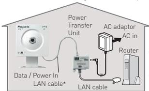
\*Use LAN cable of length 30m [98 feet 5 inches] or less to connect the camera and the power transfer unit.
